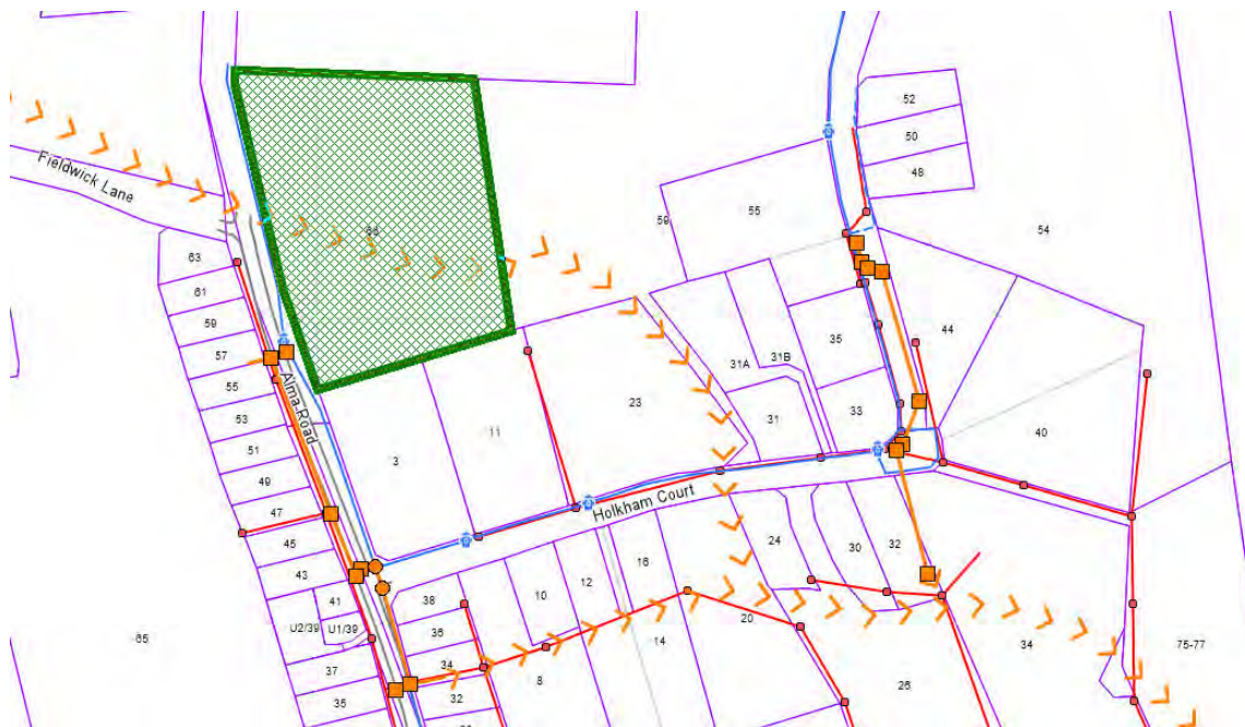
Figure 4 – Services (mains water shown by blue line; sewerage shown by red line; stormwater shown by orange lines and arrows) (source: Council's Geographic Information System)
