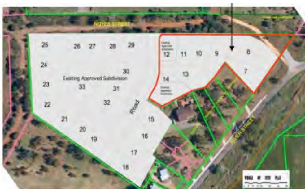
Figure 4: The existing Plan of Subdivision showing the lots to be consolidated under this application (lots 7-14) outlined in red (from the application documents). Not compass oriented.
