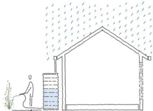
3-5kL rainwater storage provided by a slimline tank, used for irrigation and toilet flushing.
